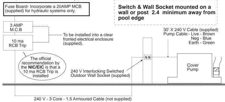
ALL WIRING TO BE PROTECTED BY 30 MA RCB COVER PUMP MUST PROTECTED BY A 10MA RESIDUAL CIRCUIT BREAKER
