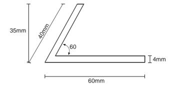
Plastic extrusion (H) are 2000 x 60 x 40 mm
