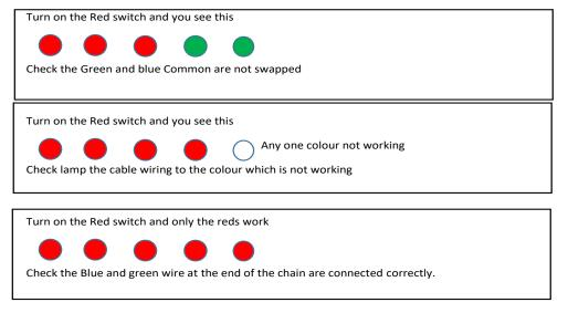
The above is a sample of what may occur if the lamps have been incorrectly wire, to sum up if you see a missing colour then check the colour cable which is not working. If all the connections are correct, then test the lamp on its own with the switch to make sure the lamp is functioning correctly
