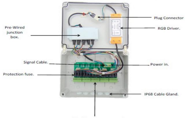
Six-Way Terminal Block for connection to the RGB Lamp.
