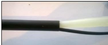
3. Put silicon sealant into the end of the heat shrink tube then heat shrink the tube to cover the cable ends, this will prevent water being pulled up through the cable to the lamp.
