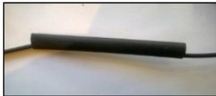
2. Place the heat shrink tube over the crimped cable and also over the black insulation
